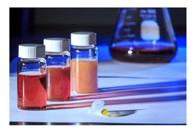
As gold ions clump together to form nanoparticles, electrons on their surface reflect light at a different wavelength -- hence the red hue. The lab tube in the foreground contains gold ions before they form nanoparticles and loaded with gene editing tools. Credit: Robert Hood, Fred Hutch
