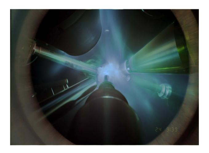
In this time-integrated photograph of an X-ray diffraction experiment, giant lasers focus on the water sample, sitting on the front plate of the diagnostic used
