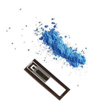
An acoustically created MOF, with the microchip that produced the high-frequency sound waves used in the process. Credit: RMIT University
