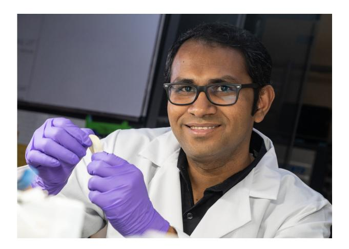
Rice University research scientist M.M. Rahman holds a flexible dielectric made of a polymer nanofiber layer and boron nitride. The new material stands up to high temperatures and could be ideal for flexible electronics, energy storage and electric devices where heat is a factor. Credit: Jeff Fitlow/Rice University
