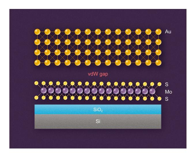
Figure 1. The method used in the study: Gold (Au) is deposited on a monolayer of molybdenum disulfide ( $MoS_2$ ), which rests upon a silicon (Si) substrate with an oxidized layer labeled  $SiO_2$ ; "vdW gap" denotes the van der Waals gap. Credit: MIPT
