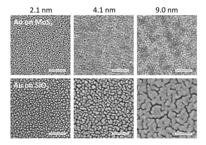
Figure 2. Gold films (Au) of varying thickness — indicated in nanometers (nm) — deposited on the conventionally used silicon dioxide substrate (SiO<sub>2</sub>, bottom row) and a molybdenum disulfide monolayer (MoS<sub>2</sub>, top row), as seen with an electron microscope. Credit: The researchers
