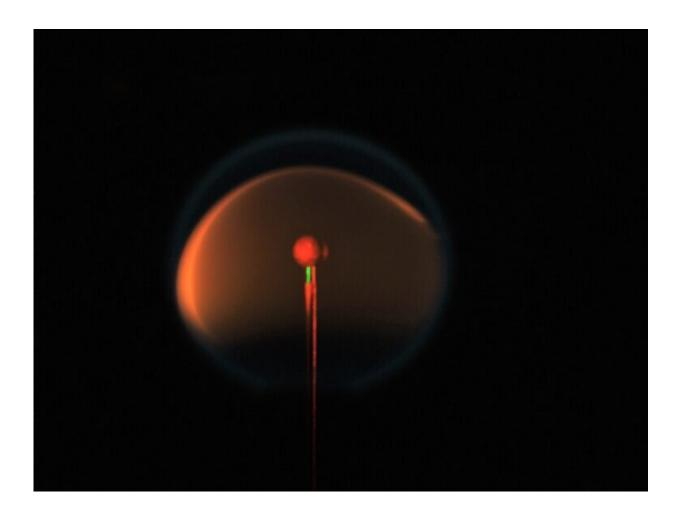
An experiment aboard the International Space Station aims to determine the true nature of soot formation during combustion. This is the spherical shape of a flame in microgravity. Credit: Richard Axelbaum/NASA
