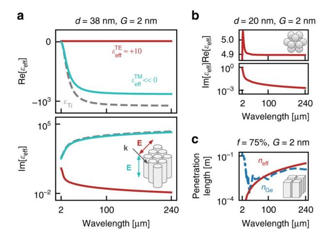
Effective permittivity of metallic nanoparticle arrays. (a) The effective permittivity of an array of titanium nanocylinders (with diameter d=38 nm and surface-to-surface separation G=2 nm) for TE (red curve) and TM (blue curve) polarized light compared to the permittivity of solid titanium (dashed curve). (b)
