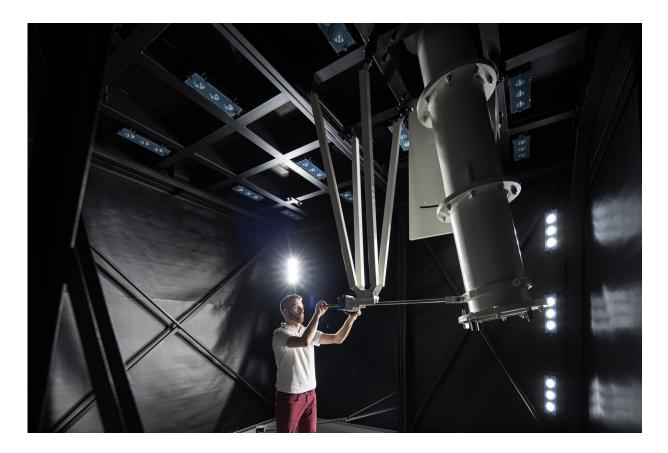
Drill platform for ExoMars rover. Credit: ALTEC
