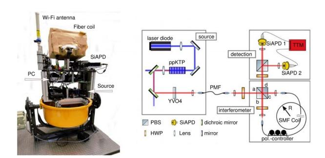
(Left) Experimental setup and (right) optical design of the fiber-optic gyroscope. Credit: Fink et al. ©2019 IOP Publishing
