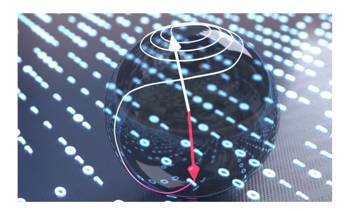
Using ultrashort pulses of light enables extremely economical switching of a magnet from one stable orientation (red arrow) to another (white arrow). This concept enables ultrafast information storage with unprecedented energy efficiency. Credit: © Brad Baxley (parttowhole.com)
