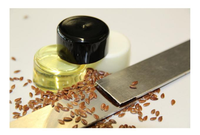
Two metal parts joined using the new, sustainably produced adhesive. Behind them: three pots containing the ingredients of the adhesive – the liquid hardener (yellow), the paste hardener (white) and the lignin organic solvent (black). Credit: Fraunhofer-Gesellschaft
