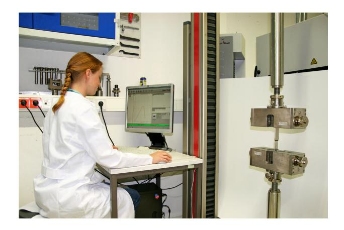
Assessing the measurement curve and determining the tensile shear strength. Credit: Fraunhofer-Gesellschaft
