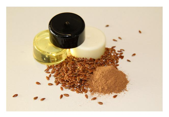
Powdered lignin and linseed. Behind them: three pots containing the ingredients of the adhesive – the liquid hardener (yellow), the paste hardener (white) and the lignin organic solvent (black). Credit: Fraunhofer-Gesellschaft
