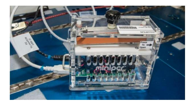
The miniPCR device, used to make multiple copies of a particular strand of DNA in space. Credit: NASA
