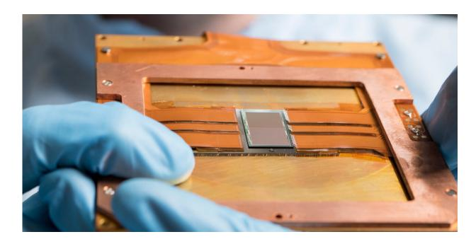
The prototype Skipper-CCD used by the researchers. Credit: Abramoff et al.
