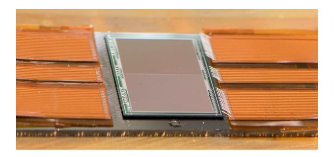
The prototype Skipper-CCD used by the researchers. Credit: Abramoff et al.
