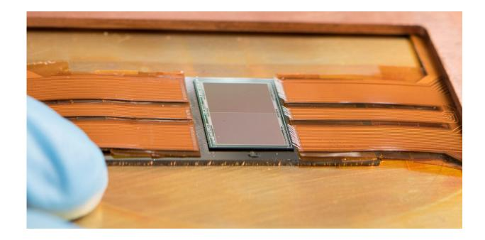
The prototype Skipper-CCD used by the researchers. Credit: Abramoff et al.
