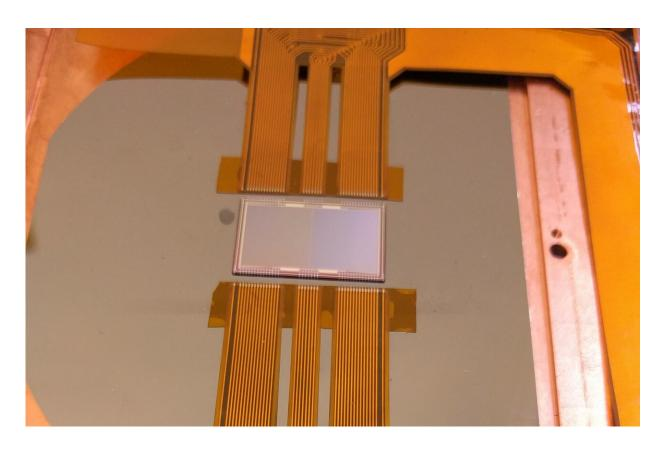
The prototype Skipper-CCD used by the researchers. Credit: Abramoff et al.
