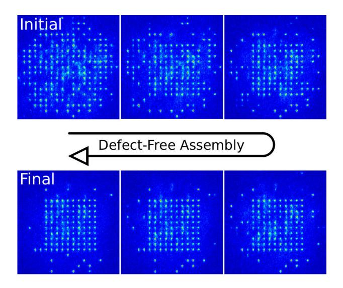
Atom pattern assembly: an initial atom distribution with defects is transferred into a defect-free 100 atom target cluster via single-atom transport. Credit: Gerhard Birkl
