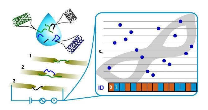
Physically unclonable functions based on single-walled carbon nanotubes. Credit: E. Burzurí
