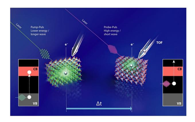
A green laser pulse initially excites the electrons in the Cu2O; just fractions of a second later, a second laser pulse (UV light) probes the energy of the excited electron. Credit: M. Kuensting/HZB
