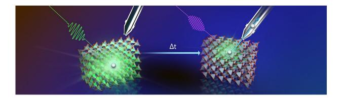
A green laser pulse initially excites the electrons in the Cu2O; just fractions of a second later, a second laser pulse (UV light) probes the energy of the excited electron. Credit: M. Kuensting/HZB
