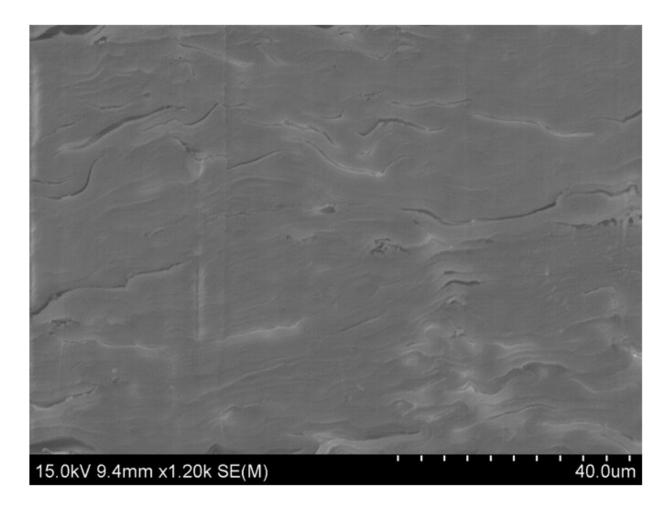
A nanoscale view of the wood's natural nanostructures shows how the fibers are closely aligned in the direction the tree grew. Credit: University of Maryland
