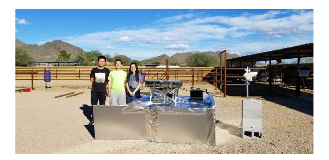
Researchers show the test device for assessing the heat-moving capabilities of the cooling wood. Credit: University of Maryland
