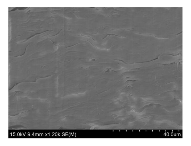
A nanoscale view of the wood's natural nanostructures shows how the fibers are closely aligned in the direction the tree grew. Credit: University of Maryland
