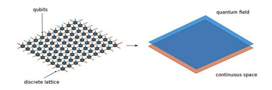
Standard tensor network states describe quantum systems that live on a discrete space, or lattice, for example an array of qubits. Continuous tensor networks, on the other hand, shrink the lattice distances until they are infinitely small and thus restore the continuity of space. This way, they can deal with quantum fields more directly. Credit: Max Planck Institute of Quantum Optics
