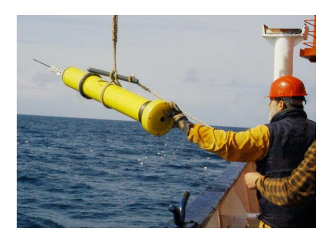
Deployment of an APEX float from a German research ship. Credit: Argo
