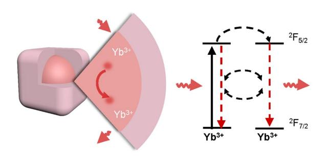
New material design and photonics technology permit over 5,000 pure ytterbium emitters to be condensed within a 10 nm crystal matrix without quenching, effectively overcoming the issue of 'concentration quenching'. Credit: University of Technology Sydney
