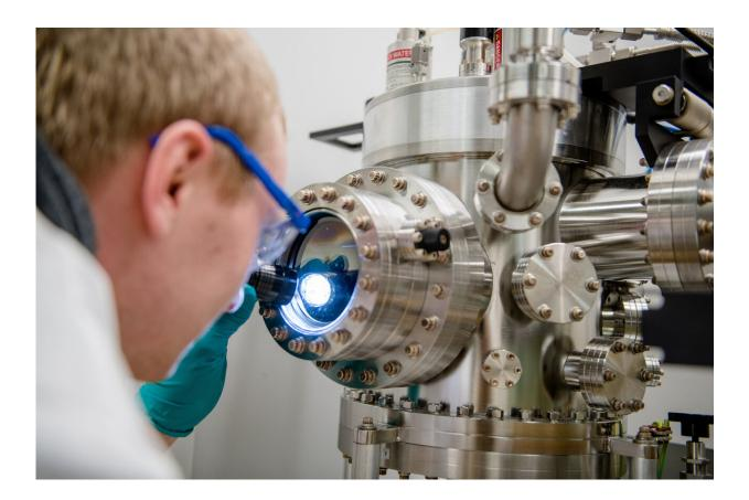
Michael Meischein in front of the sputter system in which nanoparticles are fabricated by co-deposition into an ionic liquid Credit: RUB, Marquard
