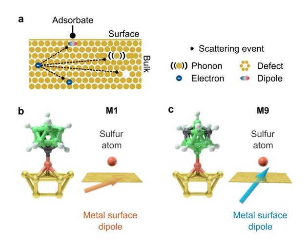
(a) When adsorbates bind to metal, they induce electric dipoles in the metal. Freely moving electrons in the metal can collide with these induced dipoles and lose their energy. (b+c) The efficiency of such a collision depends on the orientation of the induced dipoles and thus on the chemistry of the adsorbate. Credit: ©: Felix Schlapp, JGU
