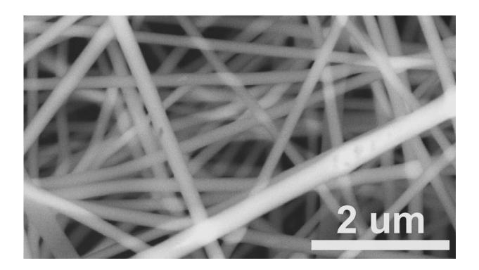
Electrospun fibers have a high surface-area-to-volume ratio, which favors surface reaction applications like catalysts, and superior mechanical properties compared with their bulk counterparts, making them less subject to mechanical failure. Credit: Argonne National Laboratory
