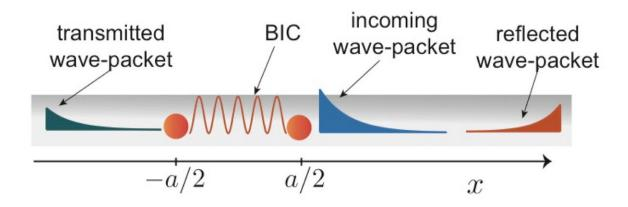
Exciting the BIC localized between two distant qubits coupled to a onedimensional waveguide: schematic for one system that permits the existence of BIC when the qubits are separated by multiple half-resonant wavelengths. Credit: Brookhaven National Laboratory
