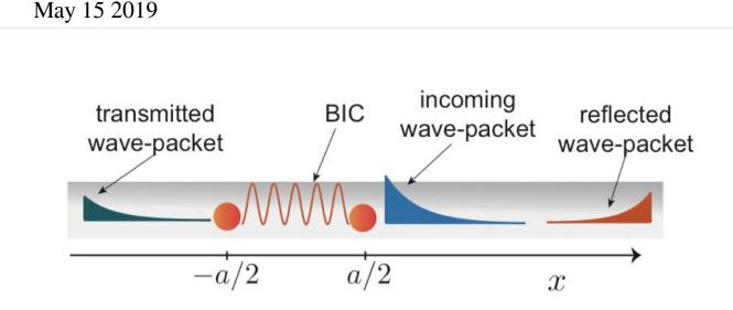
Exciting the BIC localized between two distant qubits coupled to a onedimensional waveguide: schematic for one system that permits the existence of BIC when the qubits are separated by multiple half-resonant wavelengths. Credit: Brookhaven National Laboratory
