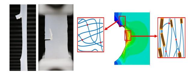
Sideways cracking in a silicone elastomer. Credit: Dr. Matt Pharr/ Texas A&M University Engineering
