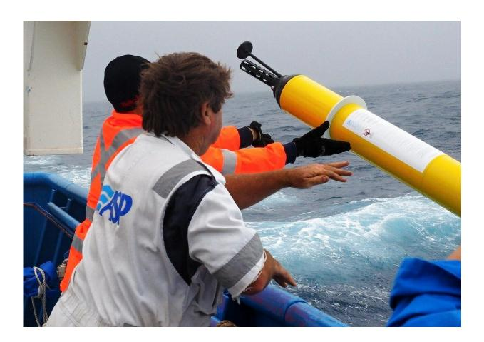
Deploying an Argo float in the Southern Ocean from the CSIRO/MNF research vessel RV Investigator. This is a file image, not connected with the current study. Credit: MNF + Stewart Wilde
