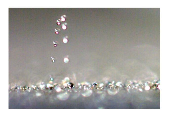
A droplet returns to a horizontal surface after jumping away. By orienting surfaces vertically, gravity can work with surface tension 'droplet jumping' as the most effective mechanism for moisture removal and heat transfer. Credit: Virginia Tech
