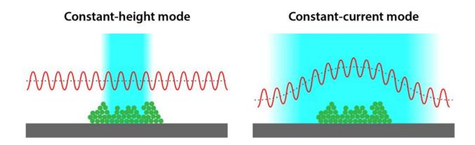
The AFM imaging of an adsorbed molecule on a substrate is usually done with the AFM tip oscillating at a constant height, where optimal imaging conditions (light blue region) are met only for the top part of the molecule. Daniel Ebeling's group uses a constant-current mode instead, in which the AFM tip closely tracks the molecule topography, allowing a complete 3D molecular imaging. Credit: APS/Alan Stonebraker
