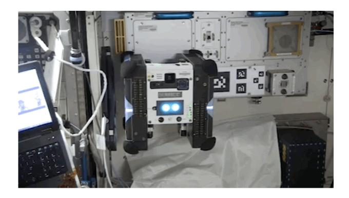
Bumble, the first Astrobee robot to power up in space, blinks while connected to its docking station in the Kibo module of the International Space Station. On
