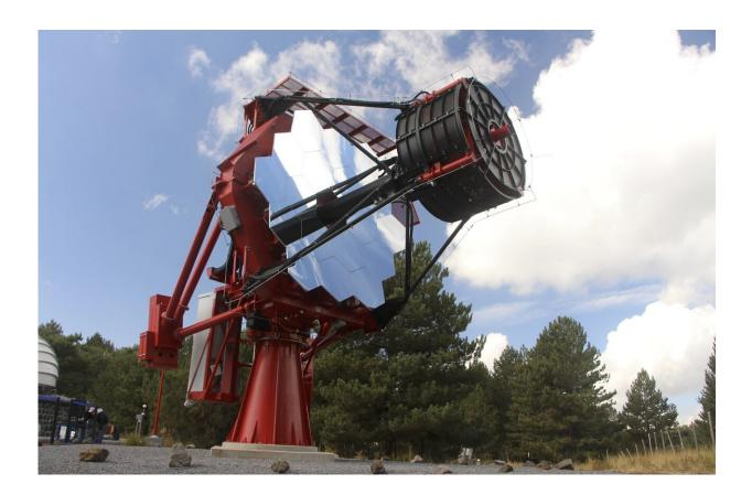
The ASTRI-Horn prototype telescope is located at the observing station of the INAF Astrophysical Observatory of Catania, in Serra La Nave, on Etna, where it was installed in 2014. The primary tassellated mirror has a diameter of 4 meters and the secondary monolithic mirror is 1.8 meters in diameter. Credit: Cherenkov Telsecope Observatory
