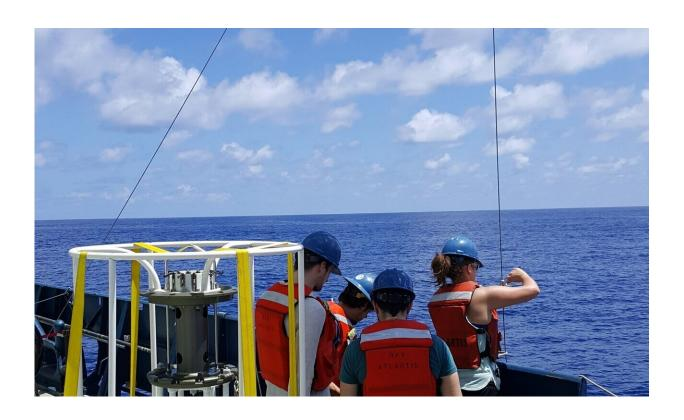
Jaclyn Saunders (far right) fixes the line on a McLane instrument that pumps large volumes of seawater in order to extract the DNA. The instrument on the left measures properties such as temperature, salinity and depth and collects smaller samples of seawater. Credit: Noelle Held/Woods Hole Oceanographic Institution
