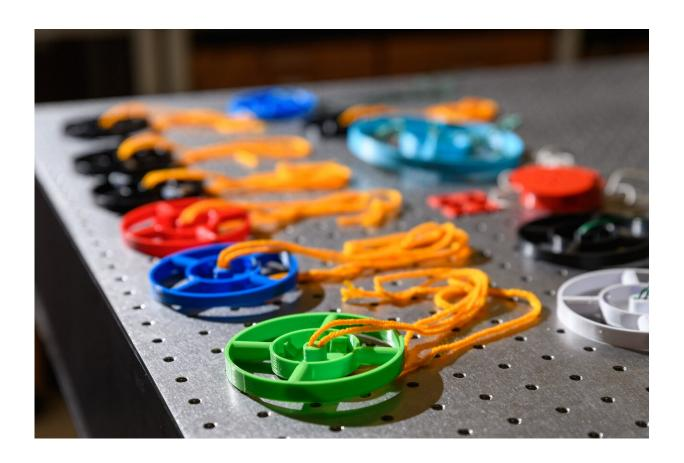
The 3D-Fuge utilizes 3D-printed disks designed to hold small vials of liquid. Simple yarn is used to spin the disks. Credit: Rob Felt, Georgia Tech
