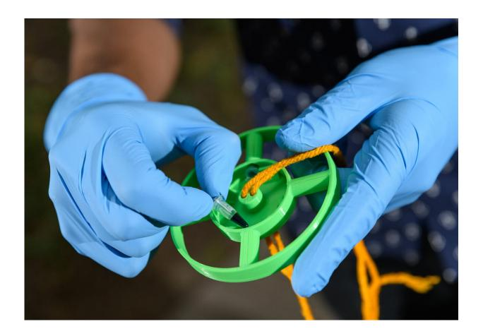
A sample vial is placed into the disk of a 3D-Fuge for separation. Credit: Rob Felt, Georgia Tech
