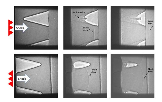
An Air Force Research Laboratory research team has developed a 3-D printed polymer-based foam structure that responds to the force of a shock wave to act as a one-way switch. These images show the material's formation of jets, which localize shock wave energy in one direction, but not the other. Credit: Air Force Office of Scientific Research
