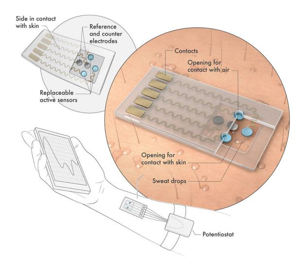
A schematic diagram of the sensor system showing how the drops of sweat are directed towards the electrodes that are coated with enzymes that can detect low
