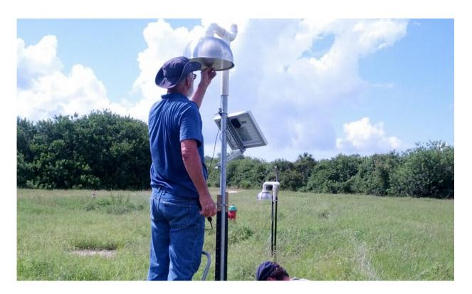
Researchers install electric field sensors in ground-based antennas that help determine the current direction that triggers lightning in the clouds. Credit: Julia Tilles
