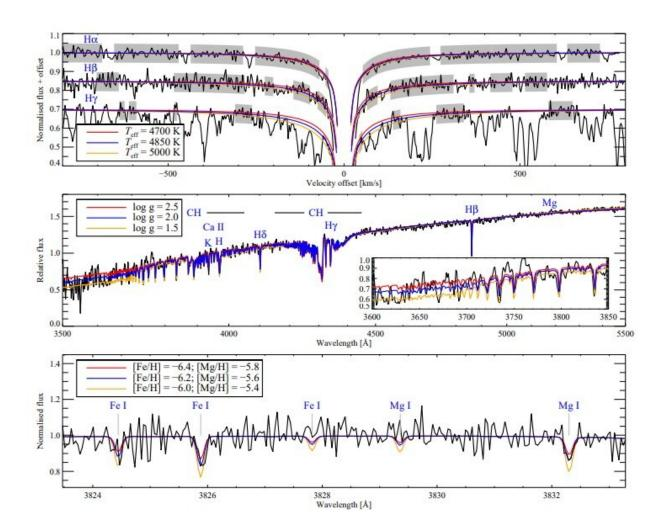
Upper panel: Fit of the effective temperature to the first three Balmer lines (labeled) in the MIKE high-resolution spectrum, compared to models at the preferred Teff = 4850 K. The lines are shown on a velocity scale centred on each line, and have been offset vertically. The grey shaded blocks represent the wavelength ranges used in the  $\chi^2$  minimisation. Middle panel: Fit of the surface gravity to the WiFeS medium-resolution spectrophotometry, with a zoomed inset
