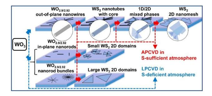
Using common ingredients for the production of tungsten disulphide, Dr. Liu and Dr. Ilie designed an evolutionary process that allows a wide range of nanomaterial morphologies to be accessed. Credit: Dr. Zichen Liu and Dr. Adelina Ilie
