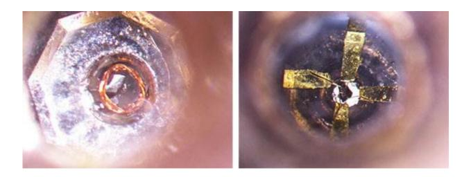
AC susceptibility and resistivity set up for UBe13 in diamond-anvil cells. Credit: Yusei Shimizu
