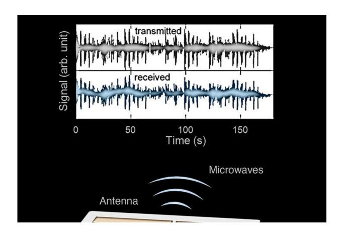
This device uses a frequency comb laser to emit and modulate microwaves wirelessly. The laser uses different frequencies of light beating together to generate microwave radiation. The researchers used this phenomenon to send a song wirelessly to a receiver. Credit: Marco Piccardo/Harvard SEAS
