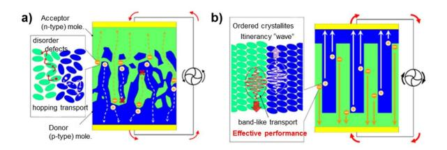
(a) Hopping conduction in disordered junction, (b) band conduction in crystalline junction. Credit: NINS/IMS
