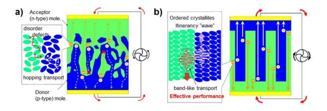
(a) Hopping conduction in disordered junction, (b) band conduction in crystalline junction. Credit: NINS/IMS
