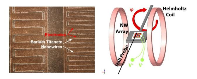
Left: Successful assembly of barium titanate nanofibers in water, post barium carbonate removal with a dilute HCl wash and suspension using citric acid and adjusting the pH to around 9, at 5 kHz and 20 Vpp. Right: Schematic of the rotating magnetoelectric measurement setup, where the angle of the array with respect to the applied magnetic field can be adjusted to explore the effects of induction on the measured magnetoelectric coefficient. Credit: University of Florida
