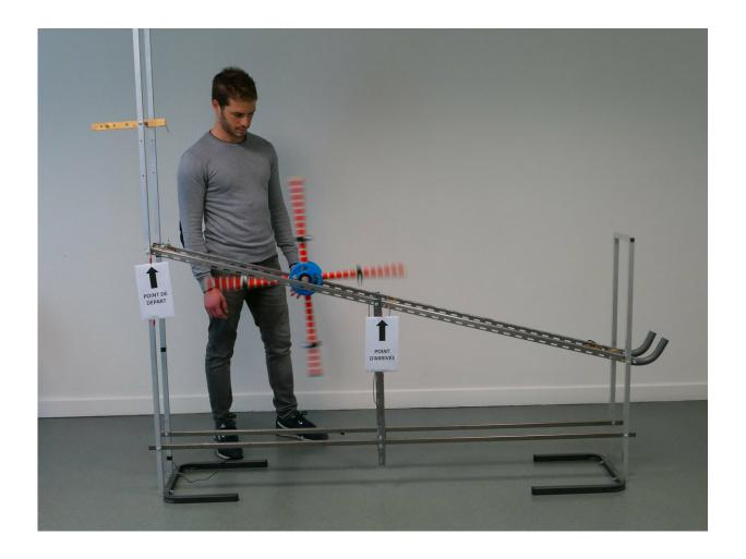
The task was to adjust the position of the weights so that the wheel rolled to the bottom of the ramp as quickly as possible. Credit: Maxime Derex
