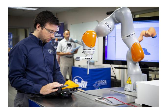
SwRI and ROS-Industrial integrated intelligent part reconstruction within the ROS2 framework to improve industrial robotics 3D image perception for path planning with way-point dense operations such as parts sanding. Credit: Southwest Research Institute
