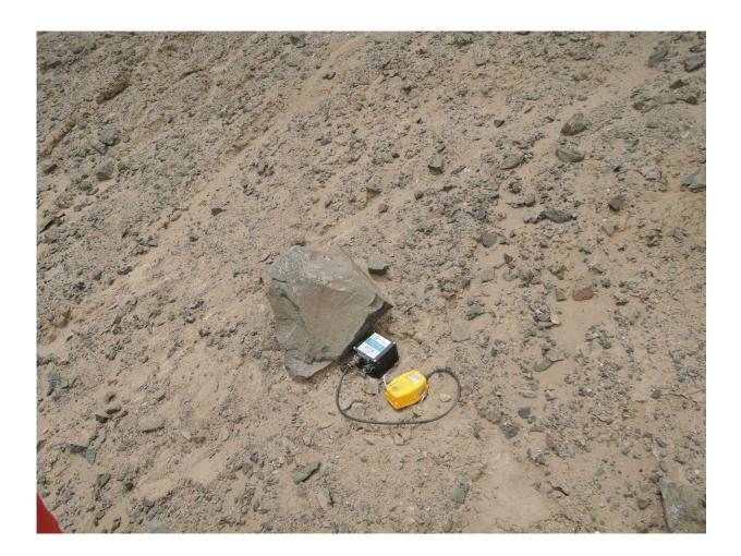
Temporarily installed geophone (yellow) with data recorder (black). Credit: C. Sens-Schönfelder, GFZ
