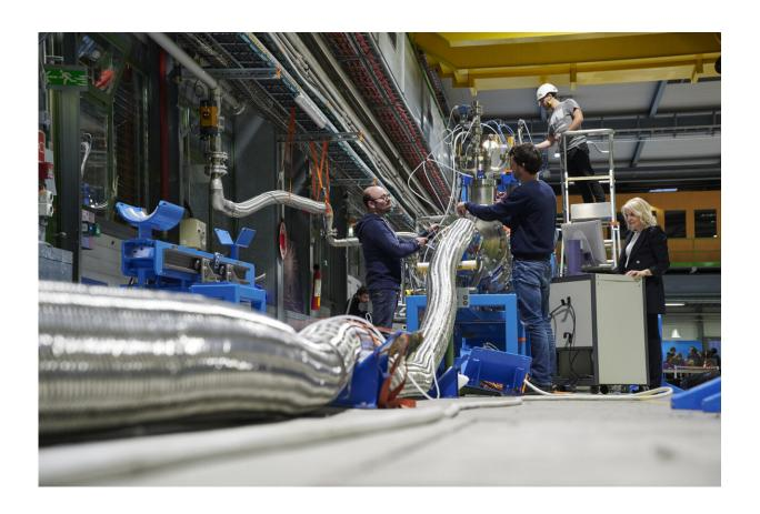
Superconducting link demonstrator system bench for the High-Luminosity LHC in SM18. Credit: © CERN
