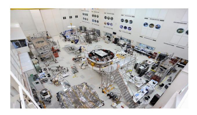
In the center of this image is the Mars 2020 spacecraft stack attached to the Spacecraft Assembly Rotation Fixture (SCARF) in the High Bay 1 clean room in JPL's Spacecraft Assembly Facility. Credit: NASA/JPL-Caltech
