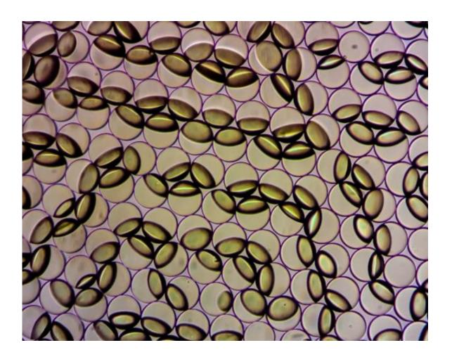
Janus emulsion droplets are captured in the process of changing form in response to the presence of contamination by a food pathogen in a lab setting. The emulsions can be viewed by the naked eye and, with the aid of a handheld sensor currently in development, can quantify the presence and amount of bacterial contamination in food. Credit: The Swager Group
