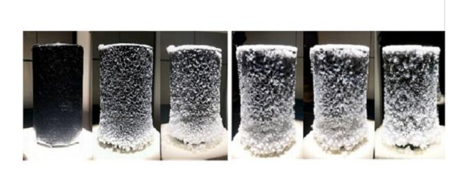
The 3-D-cup-shaped solar evaporator at increasing time intervals (l-r) at 0, 24, 48, 72, 96 and 120 hours. Credit: King Abdullah University of Science and Technology
