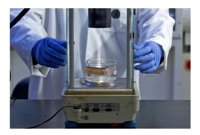
A self-cleaning device made of wood aims to make small-scale desalination more practical. Credit: John T. Consoli/University of Maryland
