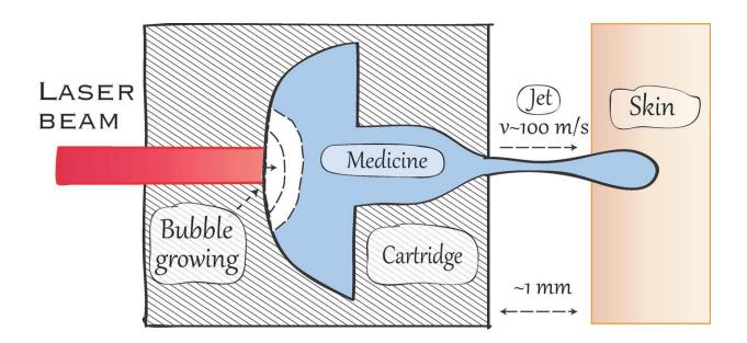
A laser heats the liquid in a microchannel. A vapour bubble grows fast, causing the liquid (containing medication or ink) to be ejected out of the channel at high speed. Credit: University of Twente
